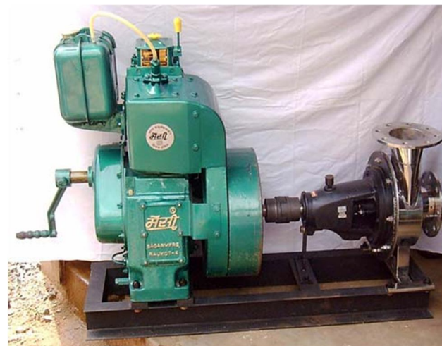
ENGINE DRIVEN PUMP SET
